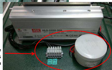
Pre-wired Power Supply And Wire Loop Connectors Inside the Station – Simplify installation
