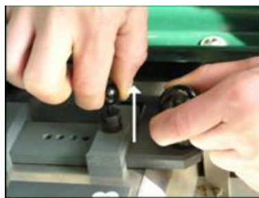
b. Lift the adjustment valve
