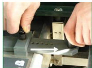
c. Slide along the adjustment rod to the desired height.
